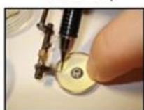
Figure 7.13: Ensuring the Shim Stays In Place
